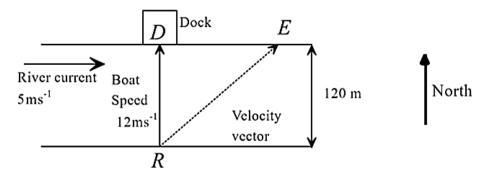
Today the current in the river is flowing at  $5 \text{ ms}^{-1}$ . From *R*, he steers the boat due north toward *D* at top speed. Due to the current, he drifts down the river and arrives at point *F*.
